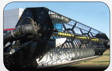
By replacing your factory reel you can add the benefit of air while keeping your header more compact, providing greater visibility.
