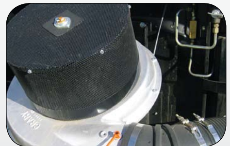
The Crary centrifugal fan provides large volumes of air through a trustworthy direct drive system.
