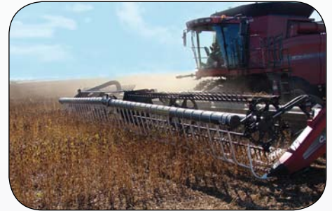
Keeping crop moving across the cutter bar is the only way to gain ground speed.
